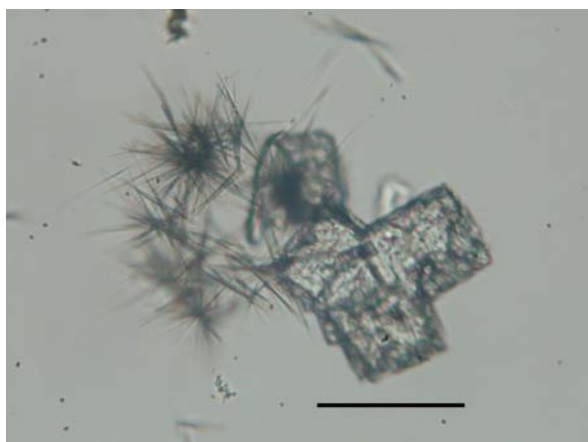
Figure 4.14. Photomicrograph of the transformation of UAD in pH 6.8 McIlvaine buffer at 37^\circ C , taken after 42 hours. Scale bar = 100 \mu m .
